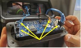
Black and red wires not used. Tuck back inside housing behind control panel.
